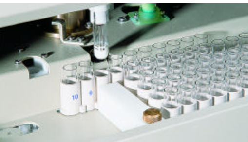
The 4C3's specially-designed cassettes move samples into position for automatic testing.
