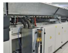
Maintenance "On-the-Fly" continues to operate while the condensation management system is being cleaned
