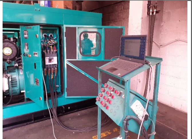
Diesel Generator Set 160 kva on during testing
