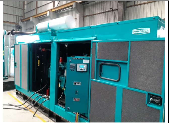
Generator Set 125 kva Testing panel display and Generator Set 200 kva during testing
