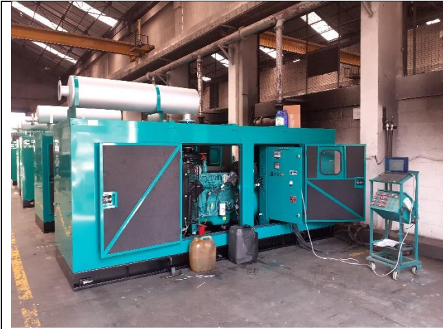
Diesel Generator Set 160 kva on during testing
