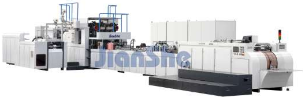
Figure 1. ZD-QFP14/18/20 Fully Auto Sheet-fed Square Bottom Paper Bag Machine.
