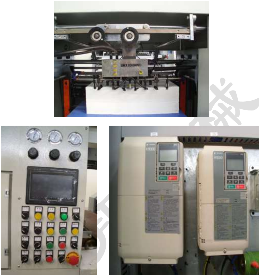
Figure 16. Components Related To Control Section
