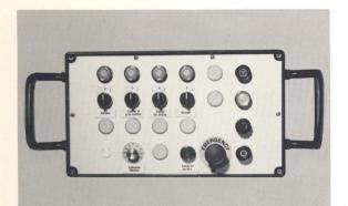
The machine is controlled from an independent cabinet which also contains the temperature regulators, etc.
