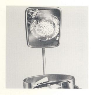
The products are put "in bulk" into the vibrator-pot. Vibration strength is infinitely adjustable. On leaving the vibrator the products are channeled into the resp. number of lanes.
