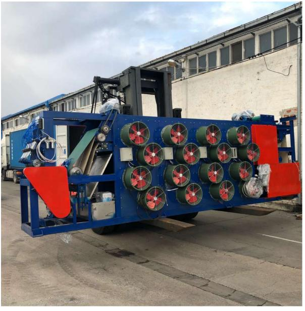
Rubber feed is pressed into rubber sheet after plasticating or mixing. This cooler can coat, cool, dry rubber sheets which are of high temperature and then be folded into a pile.
