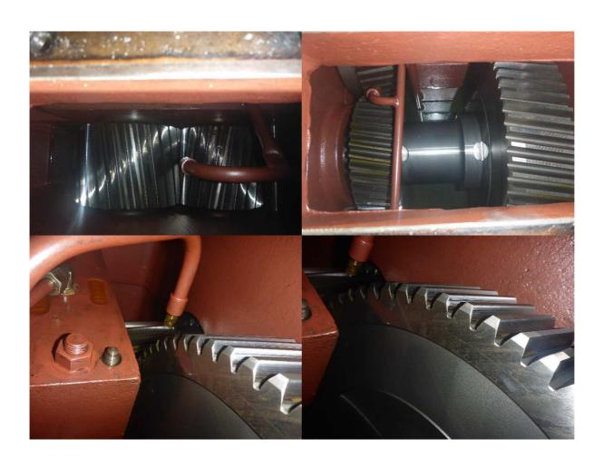
The torque limiter coupling has no identity plate of setting stamp but appears to be in good condition.
