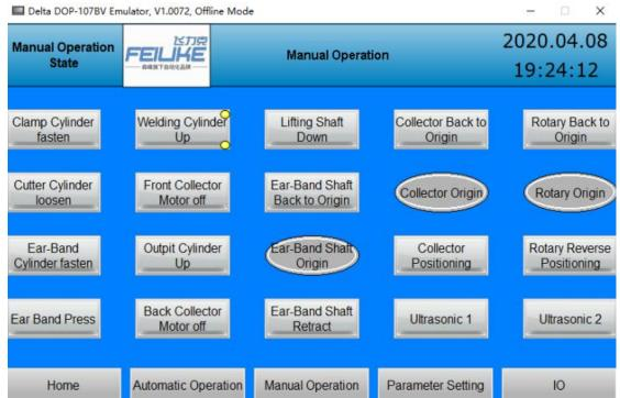
A. Welding cylinder up: Control welding head up and down.
