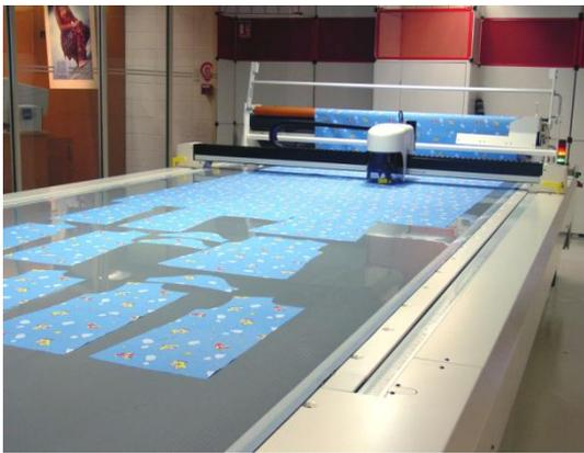
The TopSpin cutting system is ideally suited to rapid, single-ply production of large quantities of pieces, even with frequent changes of fabric.
