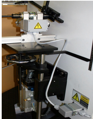
Figure 4-18: Electrical connection via plug
