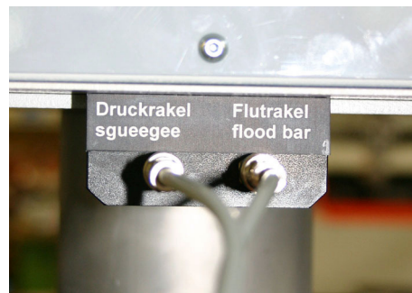
Figure 4-3: Compressed air connections for squeegee and flood bar
