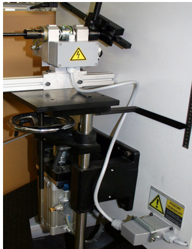
Figure 4-22: Electrical connection via plug (similar to illustration)
