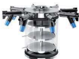
Standard chamber with 8 port manifold
