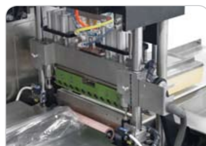
Cross seal station.
