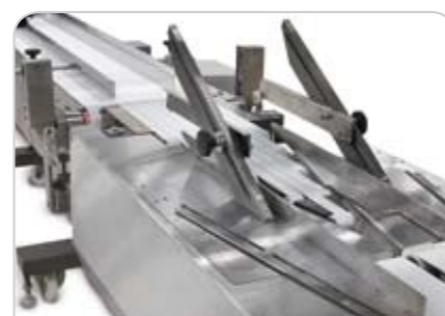
Belt type in-feed conveyor.
